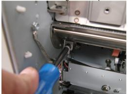
4. Remove the E-clips (2) from the Shaft.
