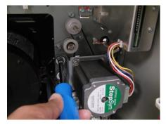
8. Remove the Timing Belt Tensioner Assembly of Motor M6 by removing (2) nuts.
