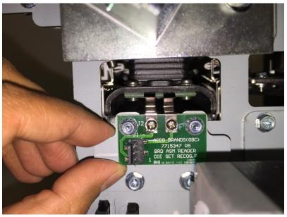
It can be set so that the top of the clips are just under the top surface of the recognition board. The spring clips will compress then the die set slides over. If the reader is set too low, the reader will not contact the recognition board. If the reader is set too high, there is a chance of mis-read and damage to clips.
