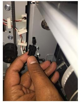
16. Disconnect the Connector for Punch Motor M10.
