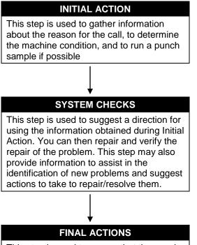
This step is used to ensure that the punch quality, the punch performance, and the punch appearance are satisfactory. It will also provide direction to help complete administrative tasks.
