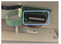
Cable 7715523 is connected at the LCD Panel.Yes-Go to Step 8No-Connect Cable 7715523
