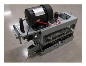
4. Disconnect the Skew Sensor Board Connector.
