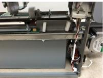
6. Remove the Screws (2) that hold the Dieset Recognition Bracket.
