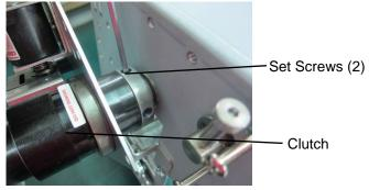
You can press down on the actuator and turn the punch shaft to orient the set screw in any direction for easy access.
