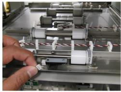
5. Remove the screw and nut for the ground strap.
