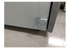
Remove the Docking Brackets from the upstream device. 5.
