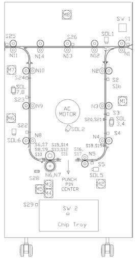
If the Punch is enabled, the transport and punch motors are started, and the Divert Solenoid SOL 1 is activated to direct the sheets into the punch path.
