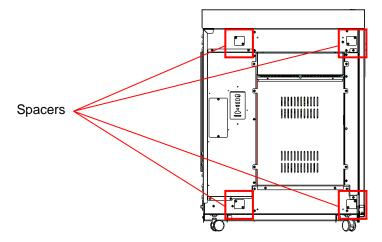
Remove the two M4 screws from each spacer. The spacers are held to the PUNCH G2 with adhesive and should remain in place. Use these screws to secure the brackets provided with the downstream device. See the Konica Minolta Installation manual for more details.
