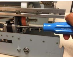
5. Adjust the belt tension such that there is a deflection of  $1\sim 2mm$ .
