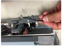
8. Remove the Steering Carriage Ground Strap.
