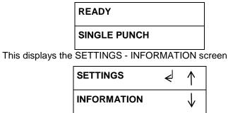
2. Press the ENTER button when the return symbol is next to the word SETTINGS to display the display the BACKGAGE/ ALIGNMENT screen.
