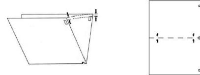
Figure 3-1 Hole Alignment on Finished Sheet
