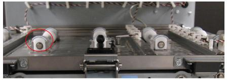
4. To adjust the Idler Panel magnetic Latches, do ADJ 1.7 Idler Panel Magnetic Latches Adjustment.
