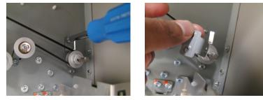
10. Remove the Upper Bypass Assembly.
