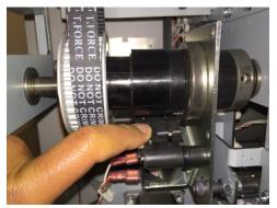
8. Remove the Clutch from the Shaft.
