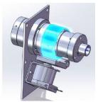
For some 230v machines, moving the stop collar towards the pulley may not expose the teeth completely. In such instances, remove the pulley off the clutch (3 sets of socket head screws and washers), see ARP 3.7 Clutch Pulley replacement.
