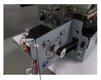
Punch Alignment Stepper Motor (M5)
