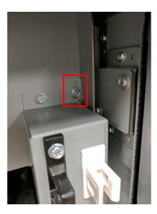
The PUNCH G2 comes with four spacers installed for the mounting of the downstream brackets.
