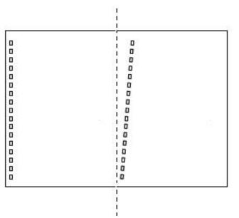
BG DP L LEFT '+' Select 1, 2, 3...etc. until the holes are parallel to the edge.
