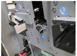
3. Loosen the Nut and Lock Screw.
