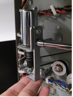
NOTE: Raising the Limiter Bracket too high will position the diverter gate higher, which will obstruct the paper flow and cause jams.
