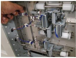
6. Disconnect the Connectors for Sensors S22, S23, & S24 at the sensor
