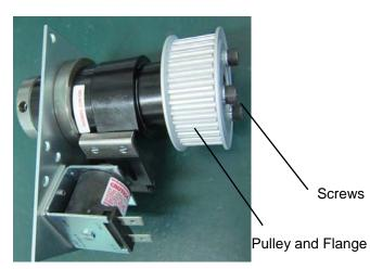
6. Remove the Lock Nut and the long M6 Screw.
