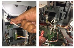
12. Disconnect the Connector for the M5 Motor Driver.
