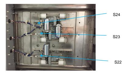
All sensors show "0" when uncovered and "1" when covered Yes- Return to the RTP that directed you here. No- Go to Step 2 5. Make sure the sensor wire is connected securely at the Sensor and at the Main Control Board. Do ARP 1.6 to remove the Rear Cover to gain access to the connector at the Control Board.
