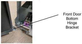
3. Screw the Front Door Btoom Hinge Bracket into the frame
