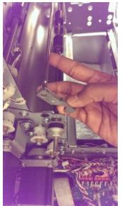
10. For the Accel Idler Panel Front Latch Assembly, slide the shaft towards the rear side to remove.
