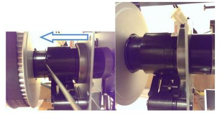
9. Move the control collar towards the pulley. By doing this the toothed hub will be exposed.
