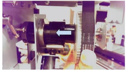
12. Manually rotate the pulley in the counter-clockwise direction by holding the pulley (viewed from rear side) to complete a punch cycle.
