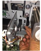
11. Disconnect the Connector for Solenoid SOL2.
