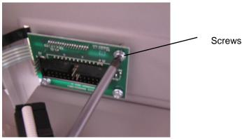
5. Remove the LCD Display.
