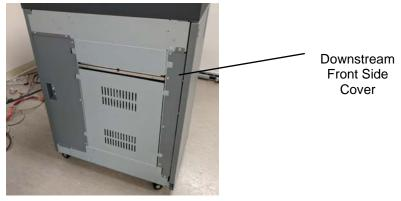
4. Remove the Downstream Front Side Cover.
