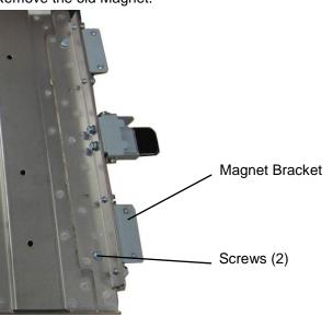
5. Place the Magnet Bracket in position and insert the Screws.
