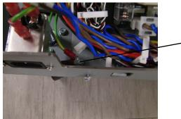
5. Remove the M4 Screws (4) from the side of the Base Frame.
