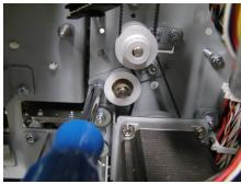
9. Remove (5) screws from the front frame that mount the Exit drive panel.
