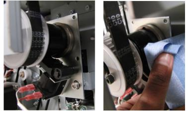
7. Inspect the collar stop and the metal insert pawl for any wear.
