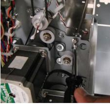
13. If you cannot remove the Entrance Drive Panel, do ARP 2.16 to remove the Idler Panel Mount Bracket (PL 2.1) from the lower position only.
