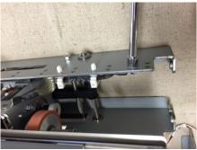
7. Remove the Ground Strap from the Wire Saddles.
