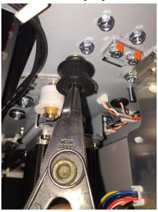
5. Remove the Timing Pulley by sliding it out.
