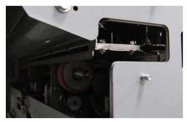
5. Check that the Steering Drive (Drive Panel Steering Sub Assembly) and the Idler Panels should be centered to the guide brackets as shown.
