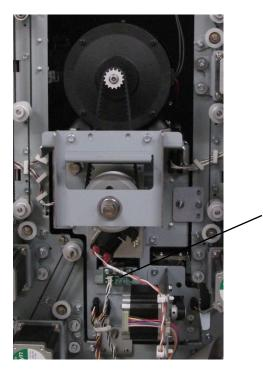
Die Set Recognition Cable 4. Remove the Screws (2) and the Die Set Recognition Board Mount Bracket.
