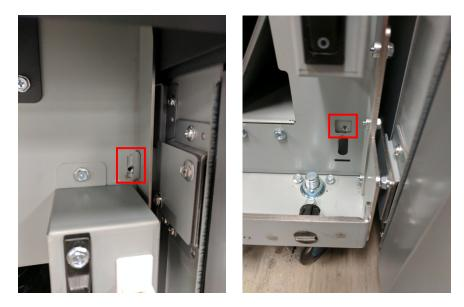
Once the brackets are aligned with the holes in the PUNCH G2, push the punch back so that it engages the alignment pins. Install item 10 in the lower right front bracket and secure the upper bracket using a M4 screw.
