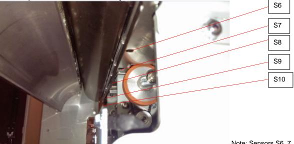
Note: Sensors S6, 7, 8, 9 and 10 are on the Skew Sensor Board
