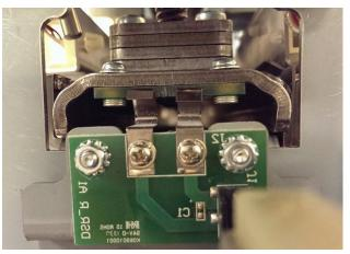
If Spring Clips are broken, Replace Dieset Recognition Reader Board. If the springs clips do not contact the Dieset Recognition Board, do ADJ 1.6 Dieset Recognition Board Adjustment.
