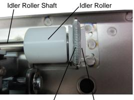
Retaining Spring Bearing Housing
