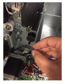
7. Slide the Pulley off the Roller Shaft.
