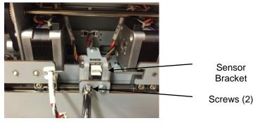
5. Remove the Sensor Sub-assembly.
