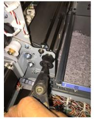
6. Remove the Belt from the Motor Pulley
