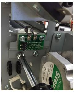
3. Insert a die set until the Dieset is about to contact the spring clips in the Reader Board.
