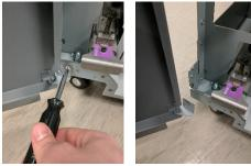
4. Lower the Door down off the pin on the Front Door Top Hinge Bracket.
