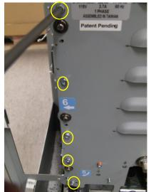
10. Remove (5) screws from the rear frame that mount the Exit drive panel.
