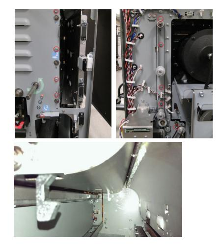
Using the Reference holes in the front/rear frame (5 holes in the front frame and 5 holes in the rear frame) and the sheet metal panel, position the drive panel to ensure the drive rollers protrude 1.5±0.5mm through the drive panel.
