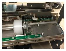
7. . Remove M3 Nuts (2) that hold the Brackets.
