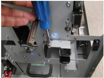
4. Remove the Rubber Cap and transfer it to the new part, if re-using the rubber cap. If a new Rubber cap has been ordered, use the new part.
