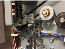
5. Remove the E-clip from the Diverter Shaft on the rear side.
