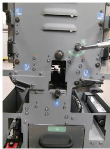
5. Use the levers (blue) to open the Acceleration Roller Idler Panel and the Exit panel.
