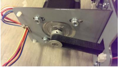
The set screws are secured tightly. Yes- Escalate to higher level No- Tighten set screw(s) and return to normal operation
