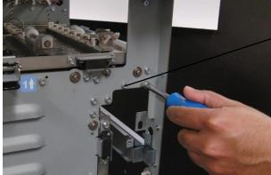
5. Remove (2) M4 screws from the rear frame.
