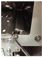
4. Remove the M4 screws (2) from the Diverter Shaft on the rear side.
