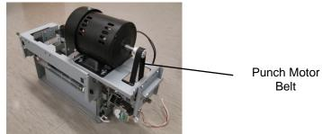
4. Do ARP 3.6 Punch Motor Belt Replacement (Timing Belt) to remove the Punch Motor Belt.
