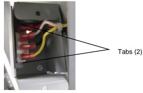
6. Note the location of the Wires (4); then disconnect the Wires from the Interlock Switch (PL 1.2).
