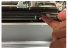
5. Remove the Nuts (3), Washers (3), and the Backage Sensor Board.
