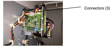
5. Remove the M4 Screws (2) and the Driver and Bracket Assembly.
