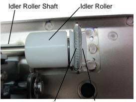
Retaining Spring Bearing Housing
