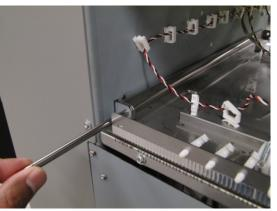
7. Remove (2) Idler panel magnetic latches from the Upper bypass assembly by unscrewing (4) screws.
