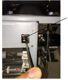
8. Remove the Socket Head Cap Screw and Split Lock Washer from the Cam and the Shaft at the front of the Punch Module.
