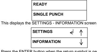
Press the ENTER button when the return symbol is next to the word SETTINGS. To display the display the BACKGAGE/ ALIGNMENT screen.
