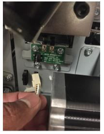
15. Disconnect the Connector for Sensors S16 and S17.
