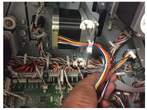
13. Disconnect the Connectors (2) for the M3 Header and the M4 Header.
