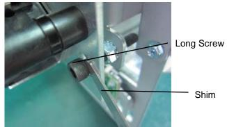
8. Use a 10 mm wrench and a 6mm Allen Wrench to tighten the Lock Nuts (2).
