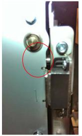
3. When the idler panel is opened and closed, you should be able to see the Idler springs extend, which will ensure proper idler roller pressure.
