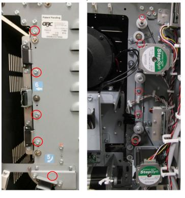
Using the Reference holes in the front/rear frame (4 holes in the front frame and 4 holes in the rear frame) and the sheet metal panel, position the drive panel to ensure the drive rollers protrude 1.5±0.5mm through the drive panel.
