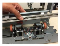
6. Remove (4) E-clips from steering drive roller shaft.
