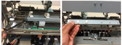
6. Unplug the Alignment Sensor Connector
