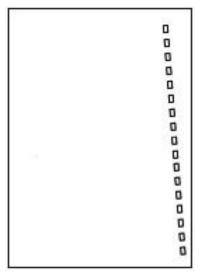
Top most hole is at correct Backgage depth, but the bottom hole is too far from the edge of the paper.
