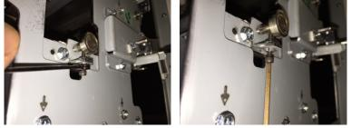
3. Rotate the Die Set Magnet counterclockwise and remove it from the Shaft.
