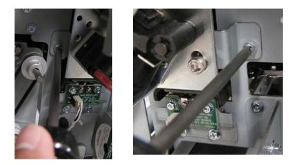
• Rotate the Clutch along with the shaft in the opposite direction (clockwise CW direction when viewed from the back) until the pins exit the sheet.
