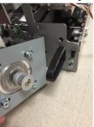
6. Pull the Alignment stepper belt in through the hole in the Frame.
