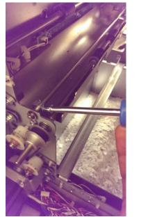
6. Remove the E-clip from the Accel Idler Shaft on the rear side.
