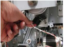
• Remove two screws that hold the Punch Clutch Bracket
