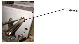
11. Pull the Shaft out through the Cams (2) and out of the Punch Module.
