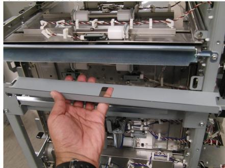
7. Use the same procedure for exit side drive roller cover by removing the corresponding screws.
