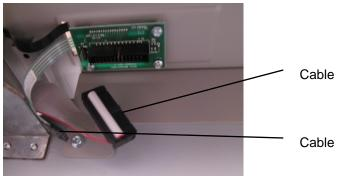
4. From the bottom side of the Top Cover, remove the Screws (3) holding the LCD Display to the Top Cover.
