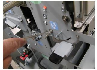
9. For the Accel Idler Panel Rear Latch Assembly, slide the shaft towards the front side to remove.
