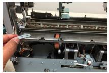
8. Transfer the Skew Sensor, Steering Idler Roller, Idler roller Cover, and all fasteners to the new Weldment.
