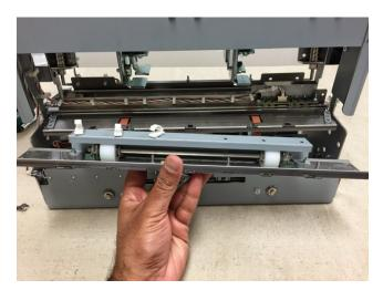
7. Be sure not to lose the spacers on either end of the drive panel.
