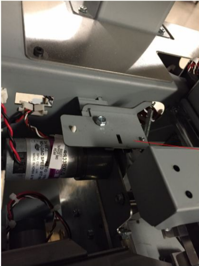
S19 is located in the tapper at the rear of the machine
