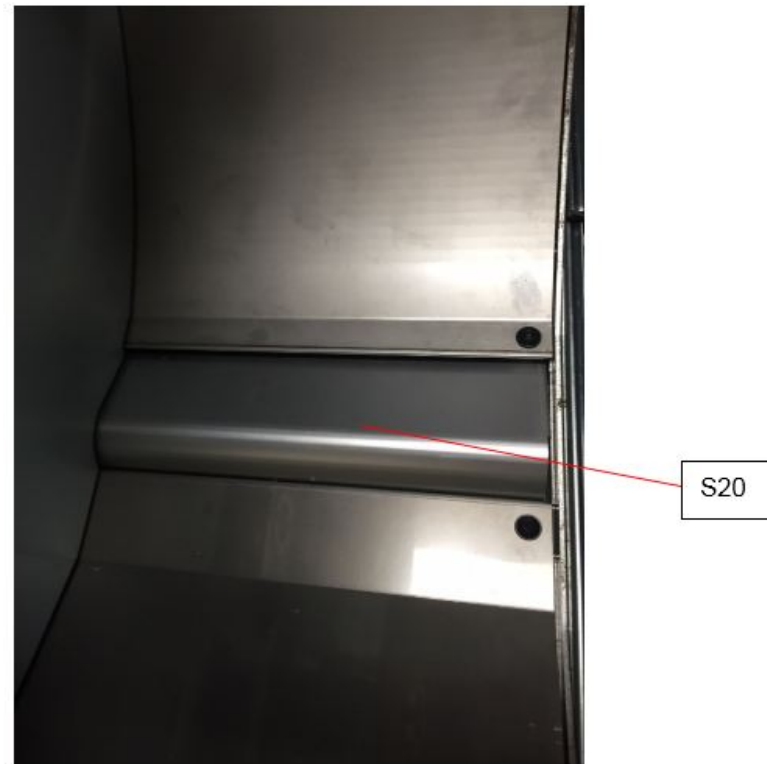
S20 is located at the bottom of the Element Feeder Assembly. It can be blocked or unblocked by pressing manually on the Slack Detect mechanism.
