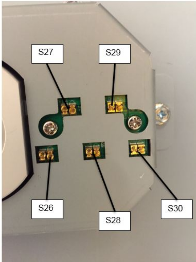
S26 through S30 are located on the front face of the element feeder spindle assembly
