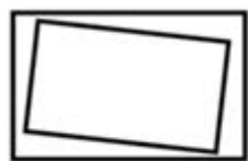
Sheet skewed along its length.
