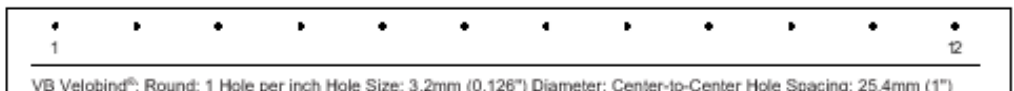
VB Velobind®; Round; 1 Hole per inch Hole Size: 3.2mm (0.126") Diameter; Center-to-Center Hole Spacing: 25.4mm (1")
