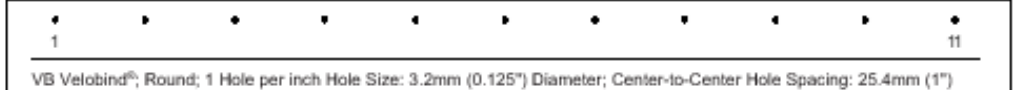
VB Velobind®; Round; 1 Hole per inch Hole Size: 3.2mm (0.125") Diameter; Center-to-Center Hole Spacing: 25.4mm (1")
