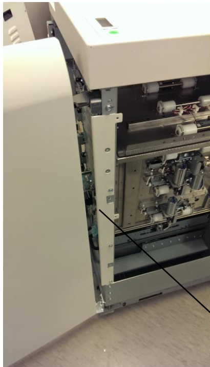
Downstream Front Side Cover
